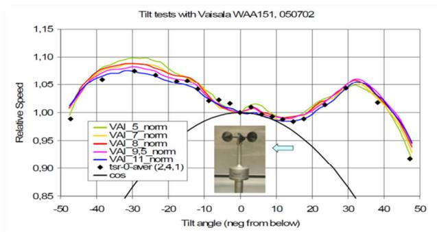
Figure 2 - Angular Response Vaisala WAA151
