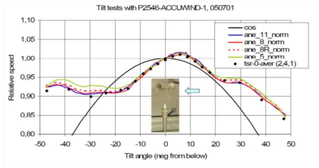
Figure 1 - Angular Response Windsensor P2546
