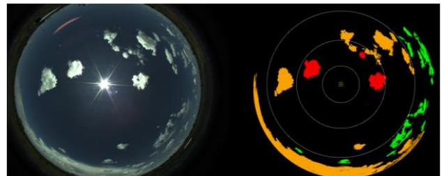
Figure 2: CloudCAM image (left) and cloud identification (right)
