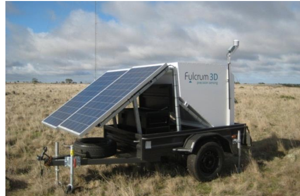
Figure 1 FS1 Sodar undergoing validation
