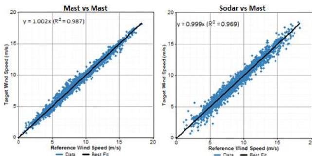
Figure 3: mast:mast (L) and sodar:mast (R) correlation result at 80m
