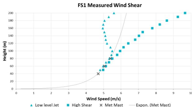
Figure 1: Examples of FS1 measured complex wind shear that would not be captured with a typical mast (but would impact wind turbines).
