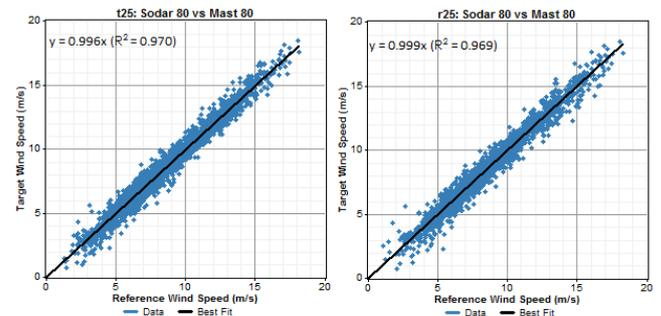
Figure 4: 80m correlation between mast and sodar ~300m apart
