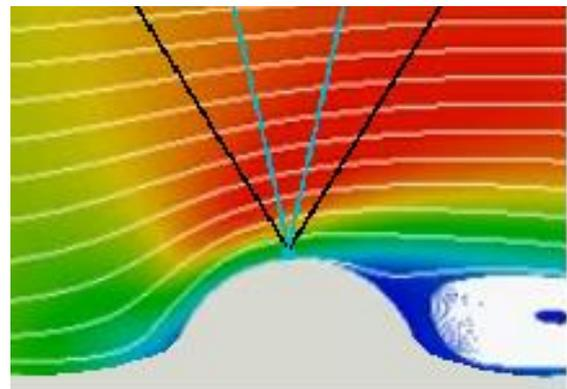
Figure 2: Wind flow over a hill showing beam locations for a 30 degree unit (black) and the Fulcrum3D FS1 Sodar (blue)
