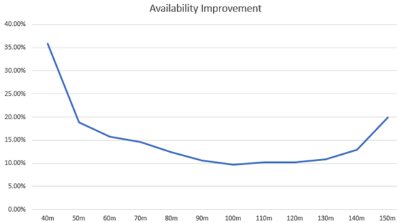
Figure 3: Availability improvement over height range through use of acoustic baffles.
